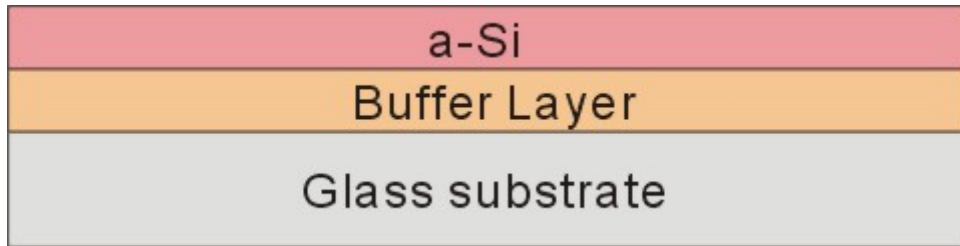
Fig. 2-4 (b) Amorphous Silicon layer deposition by PECVD system
