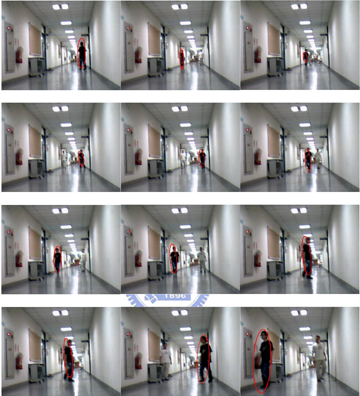
Figure 4.5-1 : Walking person tracking results of spatial-color mean-shift tracker1 with PCA scale method. Shown are frames 83, 358, 409, 494, 513, 598, 655, 689, 733, 854, 914, and 1000.
