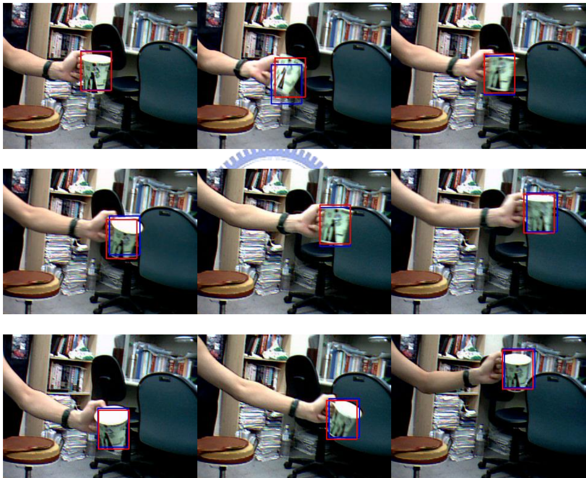
Figure 4.4-10 : Cup tracking results of spatial-color mean-shift tracker 1 with rg feature and weighted-background information in 3.6. Shown are frames 4, 45, 63, 69, 81, 105, 166, 243, 364. (red: tracker 1 with rg feature and weighted-background information, blue: tracker 1 with rg feature only)
