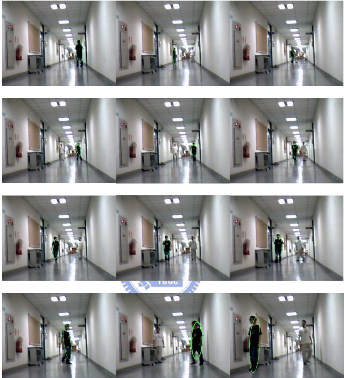
Figure 4.5-2 : Walking person tracking results of spatial-color mean-shift tracker2 with PCA scale method. Shown are frames 83, 358, 409, 494, 513, 598, 655, 689, 733, 854, 914, and 1000.
