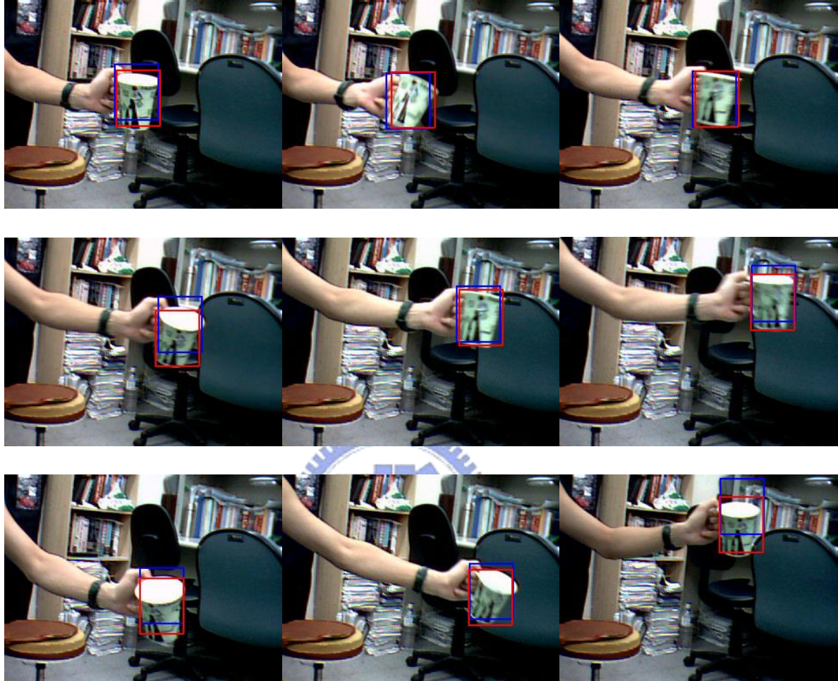
Figure 4.4-13 : Cup tracking results of spatial-color mean-shift tracker 2 with rg feature and weighted-background information in 3.6. Shown are frames 4, 45, 63, 69, 81, 105, 166, 243, 364. (red: tracker 2 with rg feature and weighted-background information, blue: tracker 2 with rg feature only)
