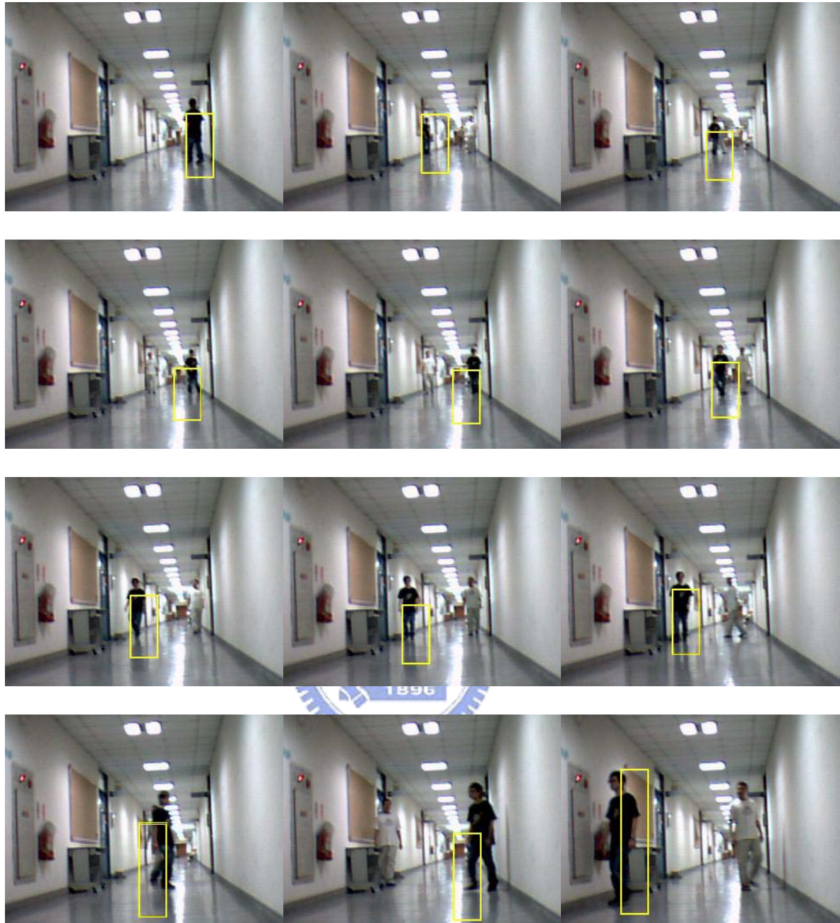
Figure 4.5-3 : Walking person tracking results of traditional mean-shift tracker with plus or minus 10 percent scale adaptation method. Shown are frames 83, 358, 409, 494, 513, 598, 655, 689, 733, 854, 914, and 1000.
