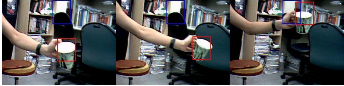
Figure 4.3-10 : Cup tracking results of spatial-color mean-shift tracker 2 with rg feature in 3.5. Shown are frames 4, 45, 63, 69, 81, 105, 166, 243, 364. (red: tracker 2 with rg feature, blue: tracker 2 with RGB feature)
