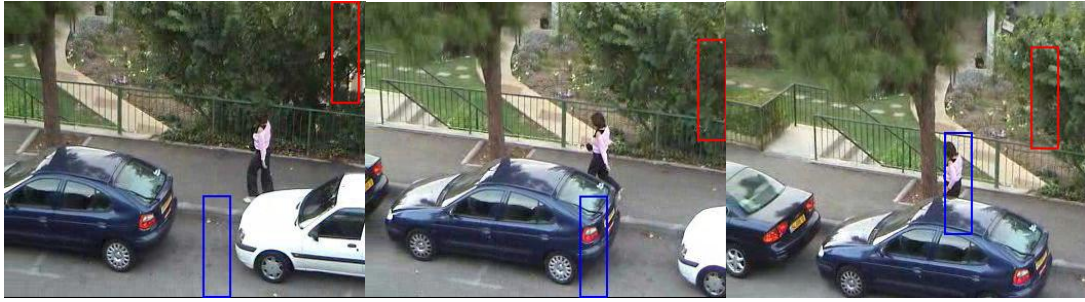
Figure 4.3-13 : Walking girl tracking results of spatial-color mean-shift tracker 1 with rg feature in 3.5. Shown are frames 28, 106, 111, 124, 130, 153, 166, 196, .220. (red: tracker 1 with rg feature, blue: tracker 1 with RGB feature)
