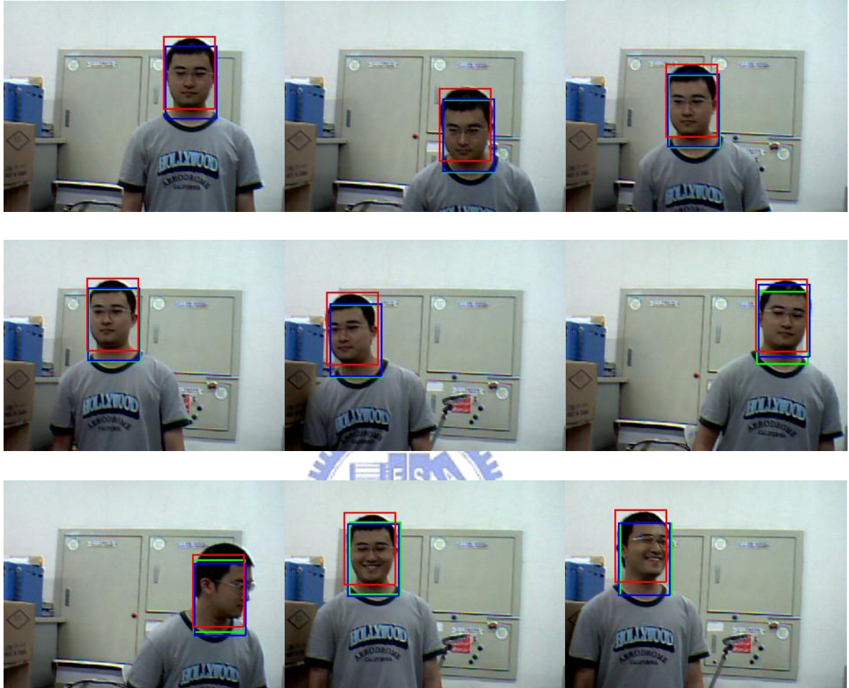
Figure 4.4-7 : Face tracking results of spatial-color mean-shift trackers with rg feature and weighted-background information in 3.6. Shown are frames 33, 93, 117, 126, 183, 256, 271, 455, 766. (red: tracker 1 with rg feature and weighted-background information, blue: tracker 2 with rg feature and weighted-background information, green: traditional mean-shift tracker)
