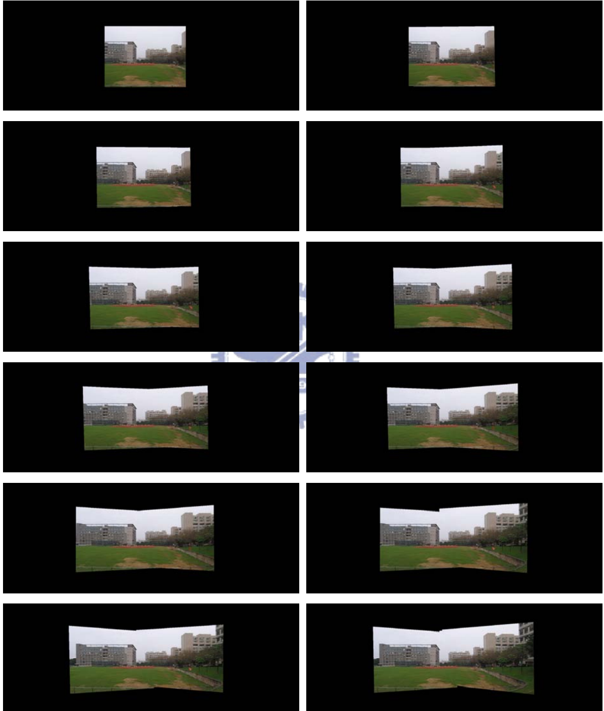
Fig 7.6 The stitching results after combining the first twelve image frames
