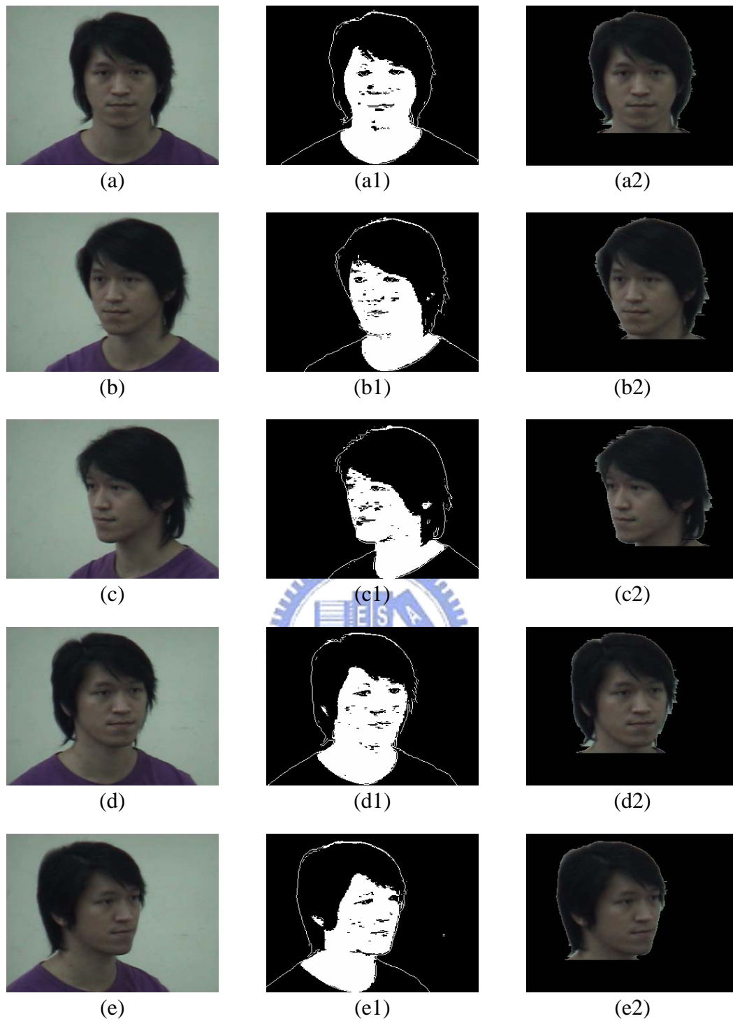
Fig. 4.9 The example 1 of head region extraction. (a)–(e) The input image. (a1)–(e1) Union of the results of YC_bC_r skin color detection and sobel edge detection. (a2)–(e2) The result of head region extraction.
