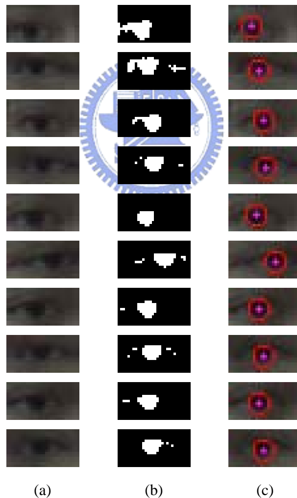
Fig. 4.14 Different face direction of iris circling. (a) Input image of eye region. (b) The intensity field. (c) Iris center located.
