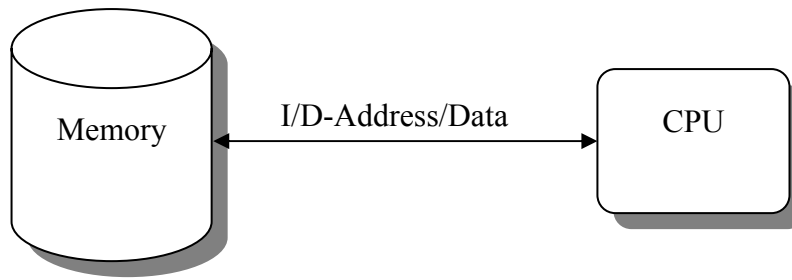
Fig. 2-3 von Neumann architecture with one bus.
