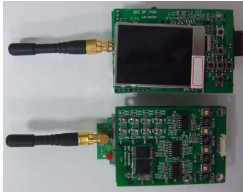
Fig.5- 14 wireless BCI using RF
