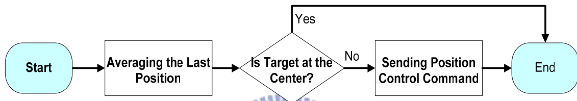
Figure 4-4 : Pan and tilt control (position control)
