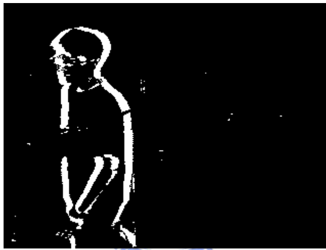
Figure 3-2 : The result of frame difference in Figure 3-1
