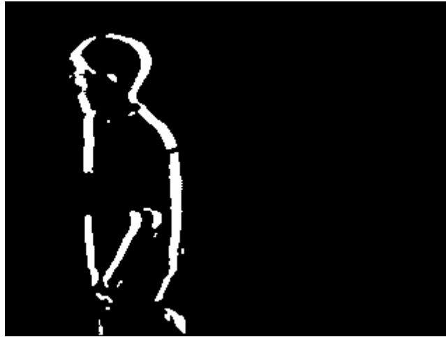
Figure 3-3 : Difference map after erosion and dilation
