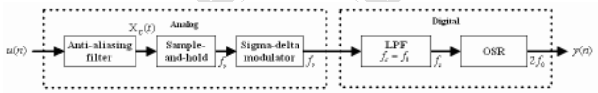
Figure 3.8: Block diagram of an oversampling \Sigma - \Delta A/D converter.
