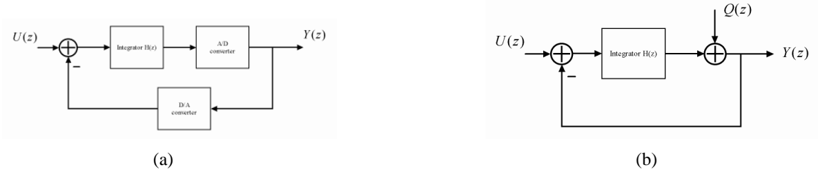
Figure 3.9: A modulator and its linear model: (a) a general SDM; (b) linear model of the SDM.
