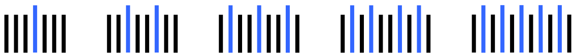
Figure 39: The optimized bus structures with different number of shield inserted in a 6-bit bus. In this figure, the black lines denote the signal wire and the grey and longer lines denote the inserted power/ground wires.
