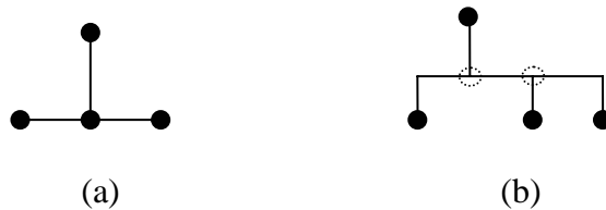
Figure 7.8 Two routing trees: (a) a spanning tree with three segments (b) a Steiner tree with the minimum number of intermediate nodes, resulting in five segments.
