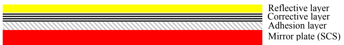
Figure 5-3 Curvature compensation by stress balance.
