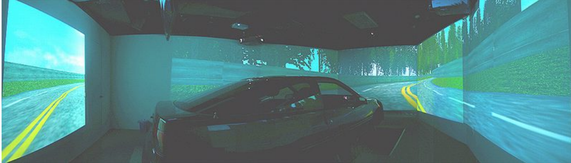
Figure 2-3: The overview of surrounded VR scene. The VR-based four-lane highway scenes are projected into surround screen with seven projectors.
