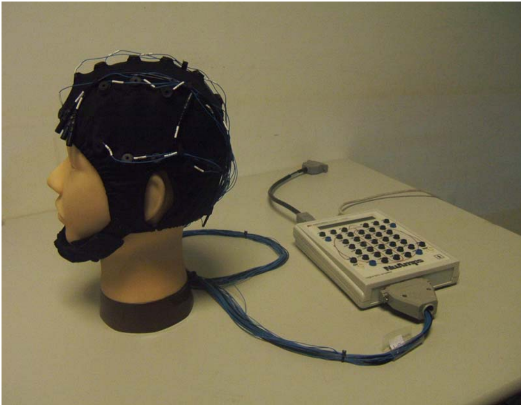
Figure 2-6: The photographic picture of NuAmps EEG amplifier and the electrode cap.
