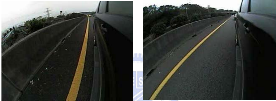
Fig. 3-14 : The different curvature of lane in (a) the lane boundary is close to the car-body. (b) The lane boundary is far to the car-body.
