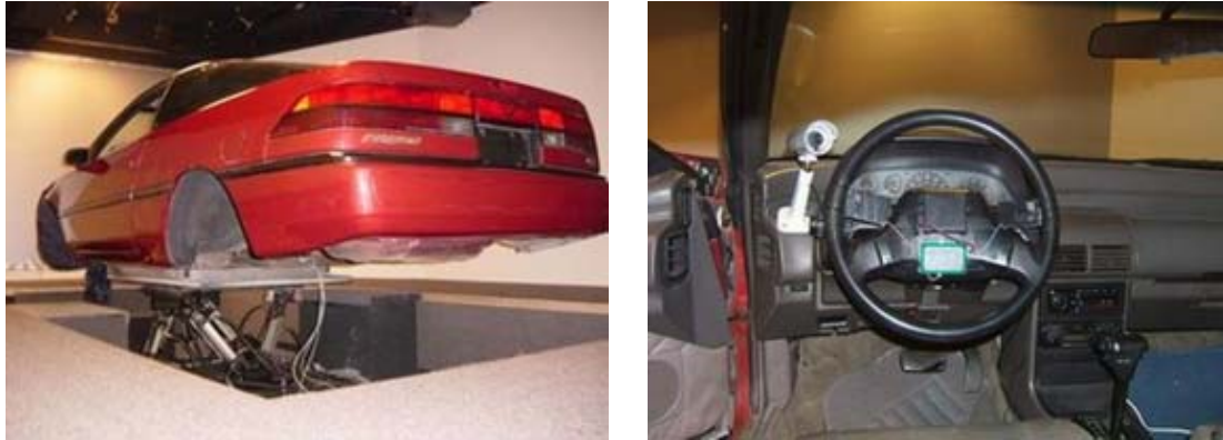
Fig. 2-2: Pictures showed the dynamic VR driving environment, in the Brain Research Center of National Chiao Tung University, Taiwan, and ROC. A real car in the 3D VR environment was showed in the left picture. The experimental setup around the steering wheel was showed in the right picture.
