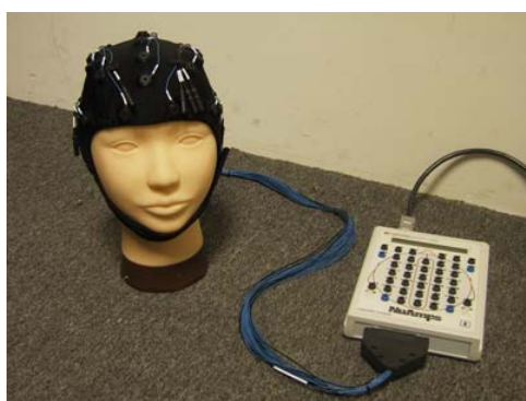
Fig. 2-6: The picture showed the setup of the physiological recording containing the NuAmps EEG amplifier and the electrode cap.
