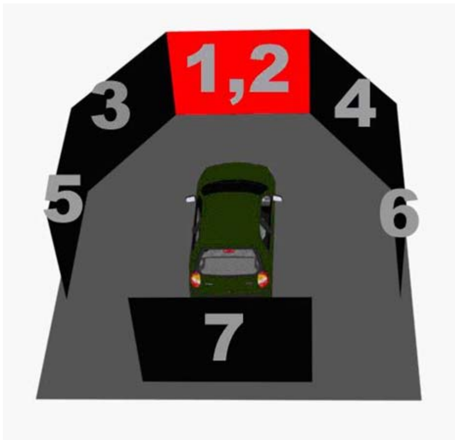
Fig. 2-3: The picture showed the configuration of the 3D surrounded scene. The 3D VR scene consisted of 7 projectors, creating a surrounded view. The frontal screen was overlapped by 2 projector frames in different polarizations, providing a stereoscopic VR scene for 3D visualization.
