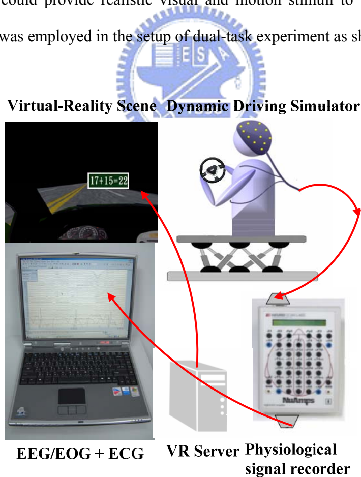
Fig. 2-1: The illustration of the experimental setup including the dynamic VR driving environment and the EEG-based physiological measurement system.
