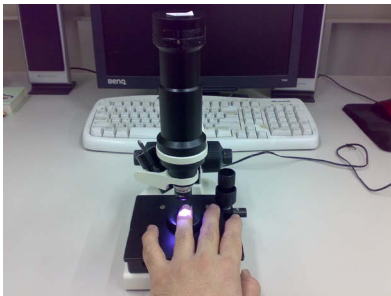
Figure 3.3 Microscope for microcirculation data collection.
