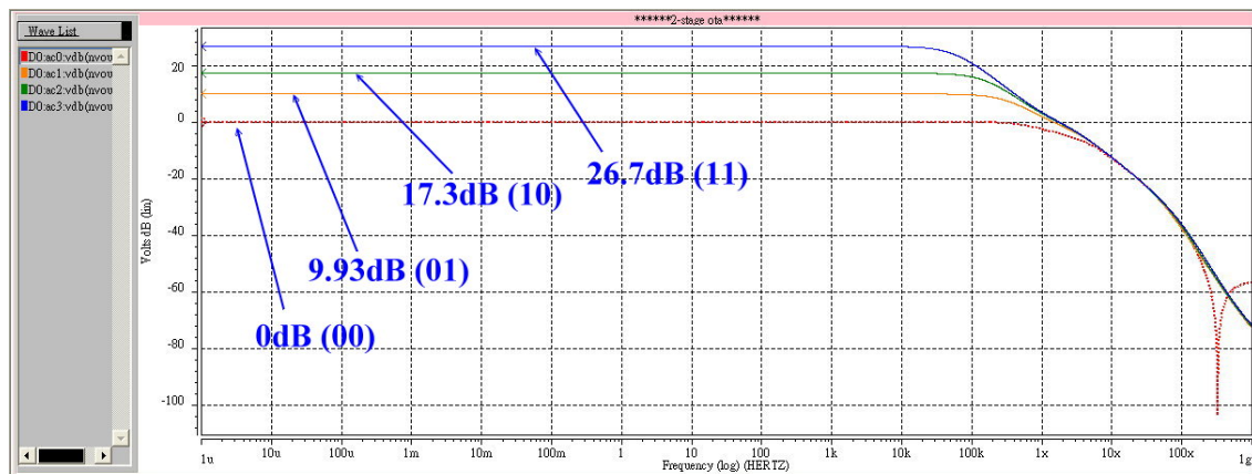
Fig. 3-22 The pre-layout simulation of PGA.
