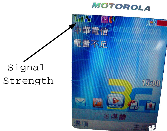
Figure 5.3: Signal Strength in a 2G System Cell Phone
