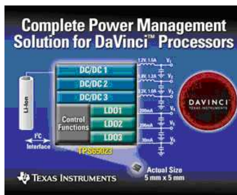
Figure 1.7: Power management IC for DaVinci technology based portable electronics [15].
