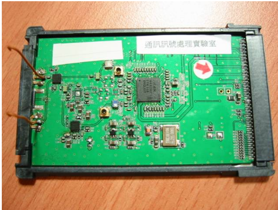
Figure 3.3: RF module on self-designed platform
