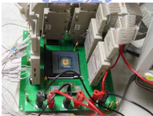
Fig 4.16 Connection between the Chip and Testing Equipments
