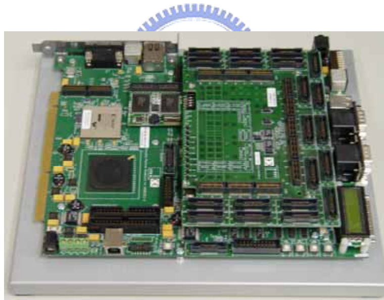
Fig 5.1 RealView Versatile Platform Baseboard for ARM926EJ-S
