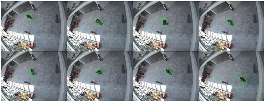
Fig. 11. Surveillance tracking results of spatial-color mean-shift tracker2 with PCA scale method (frames 3, 24, 32, 51, 59, 286, 318, and 353).
