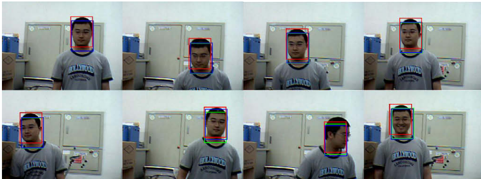
Fig. 3. Face sequence of frames 33, 93, 117, 126, 183, 256, 271, and 455. (Red: tracker 1, blue: tracker 2, green: traditional mean-shift tracker). (For interpretation of the references to color in this figure legend, the reader is referred to the web version of this article.)
