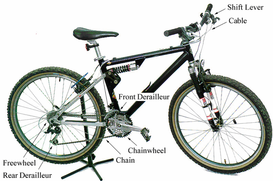
Fig 1.1 Bicycle derailleur system [1]
