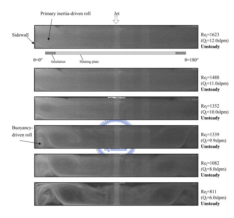
Fig. 4.46 Unsteady side view flow photos taken at the cross plane  $\theta = 0^{\circ}$  & 180° for various jet Reynolds numbers at Ra=60,160 ( $\Delta T = 10^{\circ}$ C) for H = 40.0 mm.
