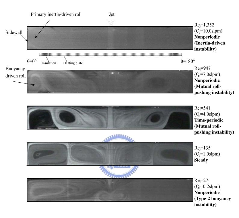
Fig. 4.82 Side view flow photos taken at the cross plane  $\theta = 0^{\circ}$  & 180° for various jet Reynolds numbers at Ra=30,065 ( $\Delta$ T=5°C) for H = 40.0 mm.
