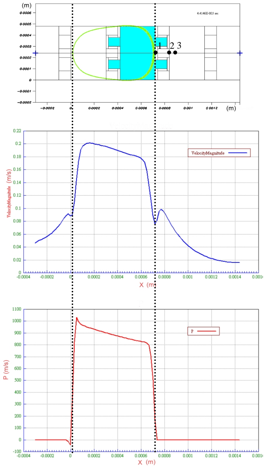
Fig. 4-4 Illustration of velocity and pressure for droplet (case 3)
