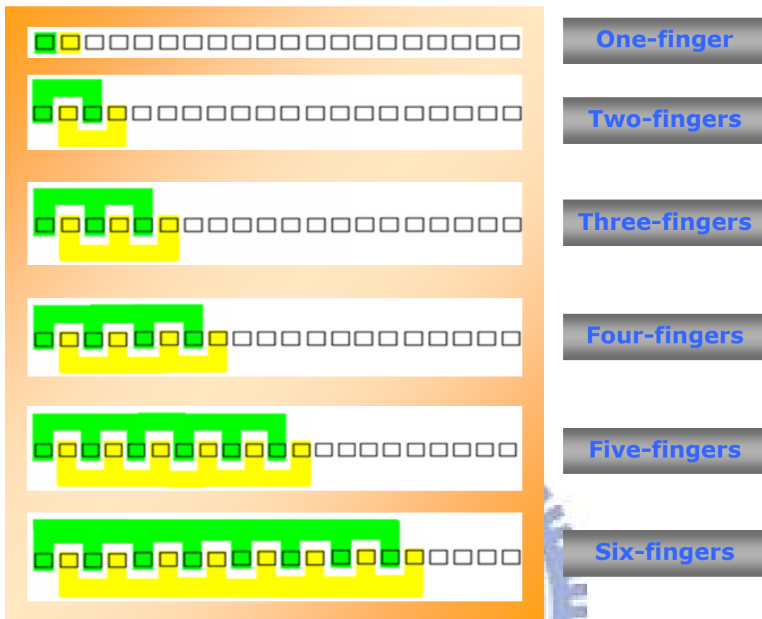
Fig. 3-2-6. Illustration of the interdigitated method of the crossstie device with more fingers
