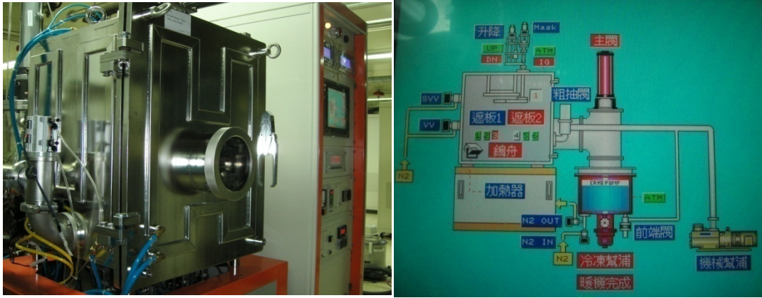
Fig.2-2: The thermal deposition instrument
