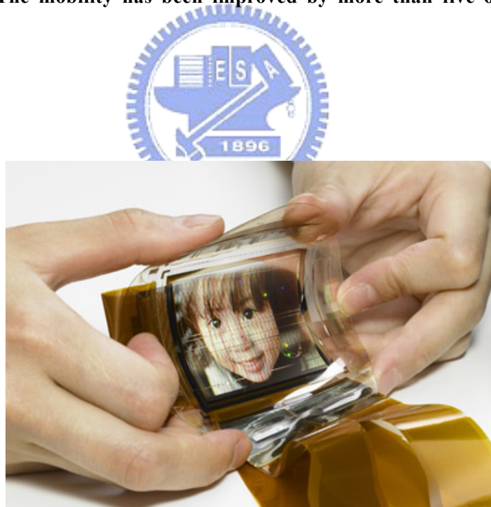
Figure 1.2 The first full-color active-matrix organic LED display on a flexible plastic substrate developed by SONY Corp.
