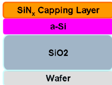
Figure 2-8the simple structure with SiN x capping layer
