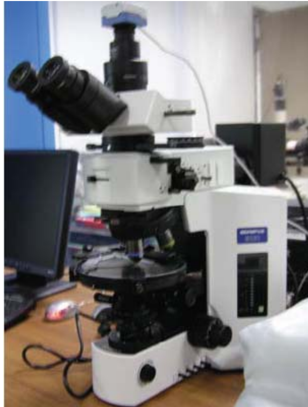
Fig. 3.5. The picture of POM Olympus BX51.
