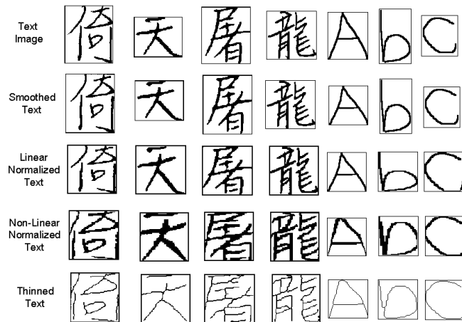
Figure 4.2: Image preprocessing on handwritten characters: (from top) original text image, smoothed text, linear normalized text, nonlinear normalized text and thinned text.
