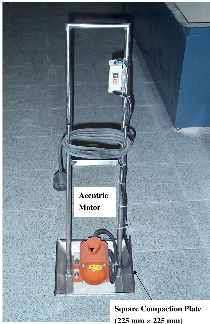
Fig. 3.6. Vibratory soil compactor (after Chen, 2003)
