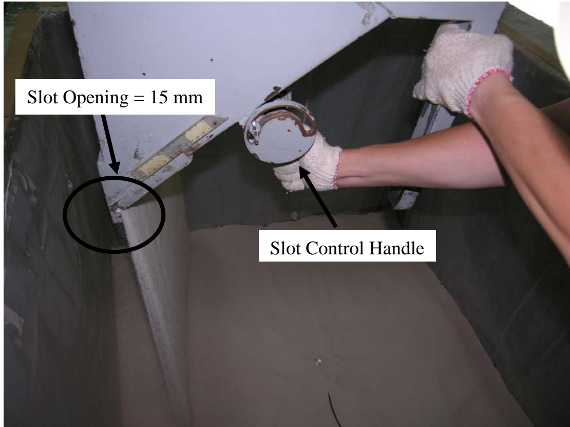
Fig. 5.3 Method to Control Slot Opening = 15 mm
