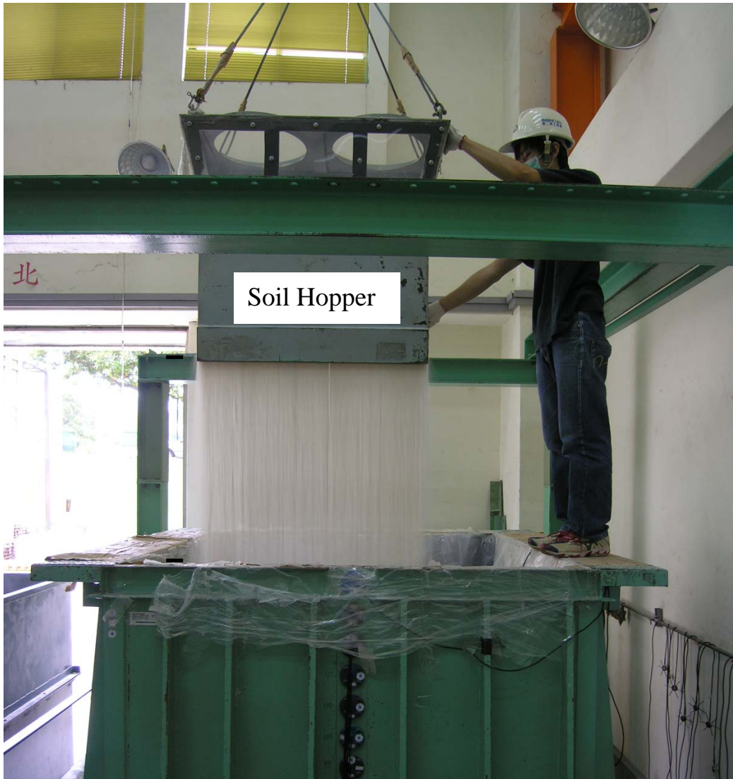
Fig. 5.4 Pluviation of Ottawa Sand into Soil Bin
