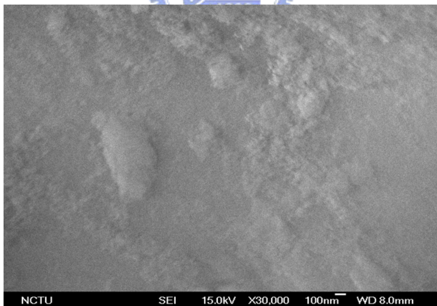
(b) Porous silica in low-k underfill material D (1:3)
