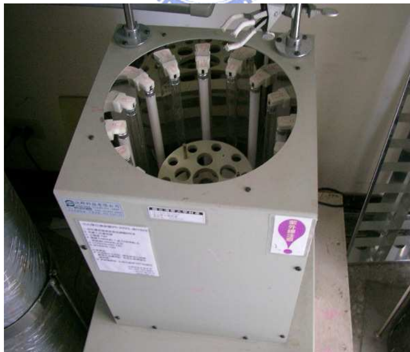
Figure 3-4. Photocatalytic reactor with 6 UV light tubes of 305 nm set around the fused-silica tubes.
