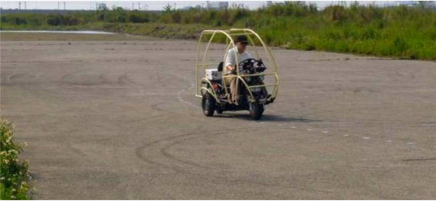
Fig. 17. Slalom test without tilting motions.
