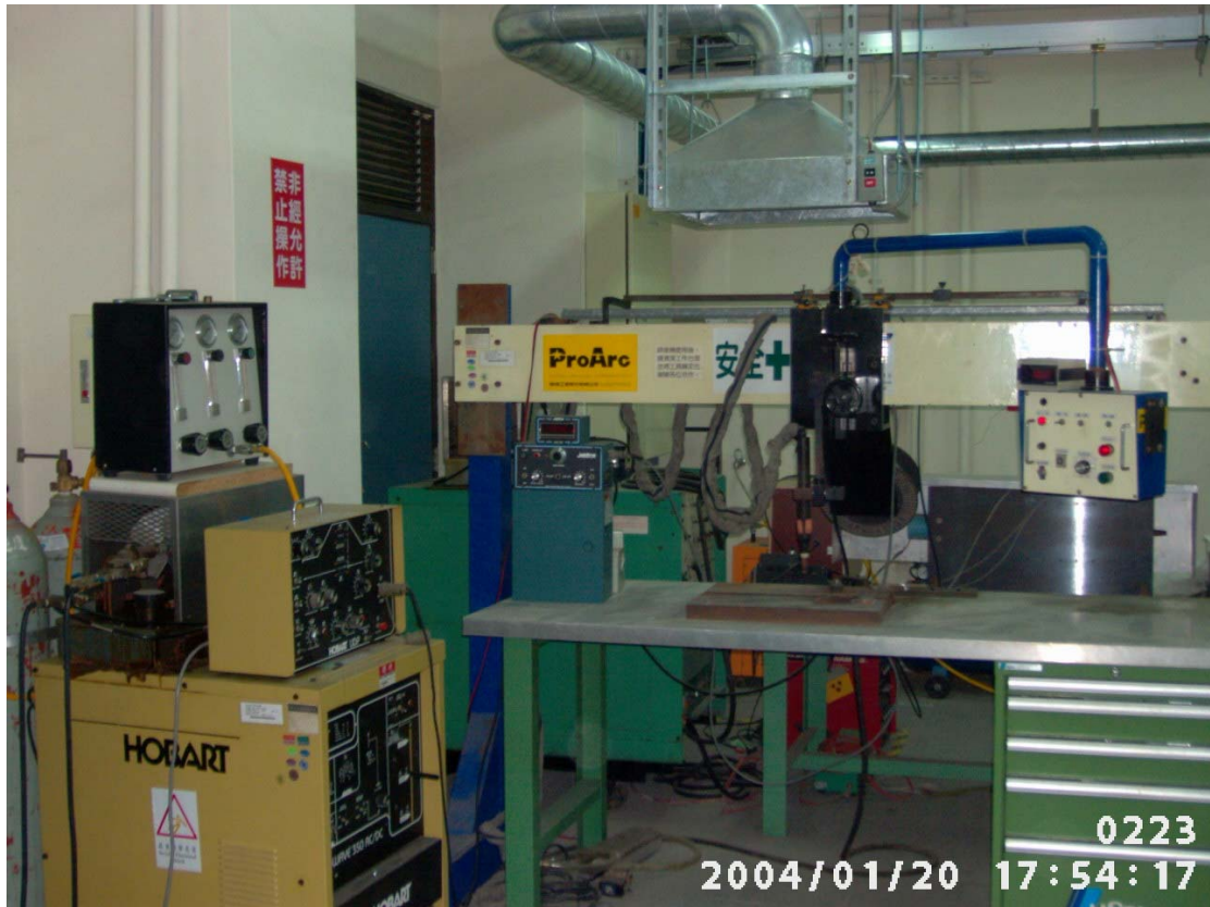
Fig. 3-1 The equipment of Autogenous GTA welder
