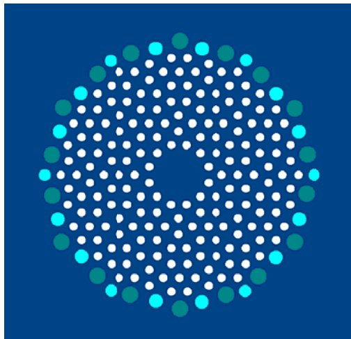
Figure 3.15: The CAD design with alternative air holes. The outer three layers are replaced by air holes with alternate radius. The distance between two different radius air holes can produce enough tolerance for over dosage and prevent membrane from crashing.
