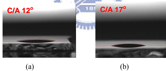
Fig. 4.3 Contact angle of red ink drop on blank BM and glass (a) blank BM (b) blank glass
