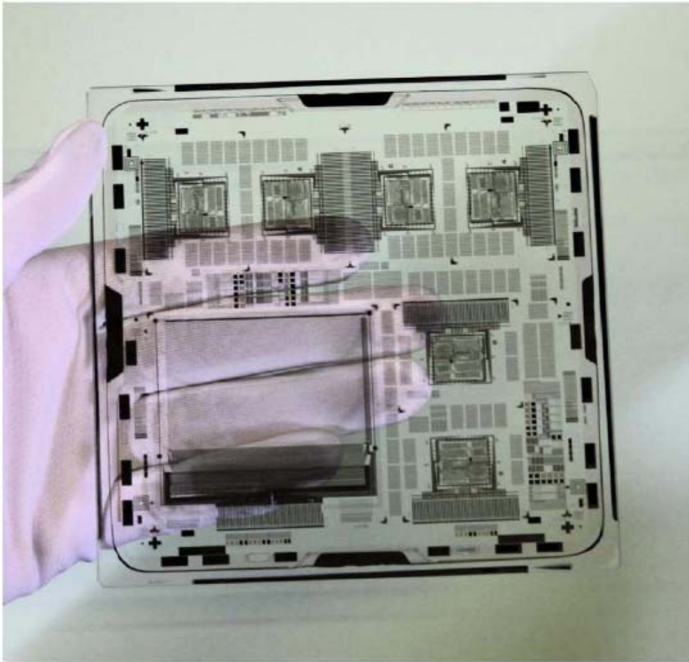
Figure 1-3 The system on glass prototype with the poly-Si TFT technology from Sharp
