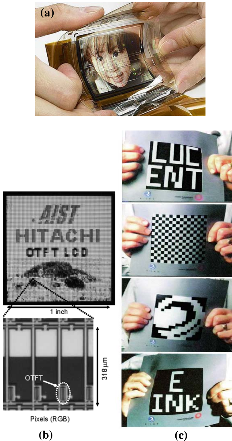
Fig. 1-1 (a) Pentacene-based array combined with light emitting diode [Sony, 2007] (b) Pentacene-based array combined with liquid crystal [Hitachi, Ltd., 2006] (c) Pentacene-based array combined with electrophoresis [National Academy of Sciences, 2001].
