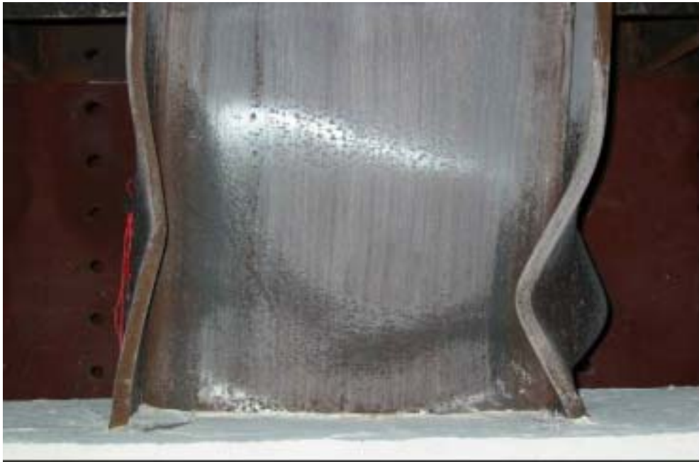
(c) 位移 10\Delta y 時( Story Drift Angle \theta_t = 4.77\% \text{ rad} , Beam Plastic Rotation \theta_{bp} = 3.43\% \text{ rad} )
