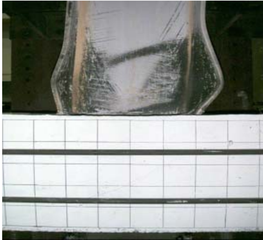
(c) 位移 11\Delta y 時 ( Story Drift Angle \theta_t = 5.25 \% \text{ rad} , Beam Plastic Rotation \theta_{bp} = 4.28 \% \text{ rad} )
