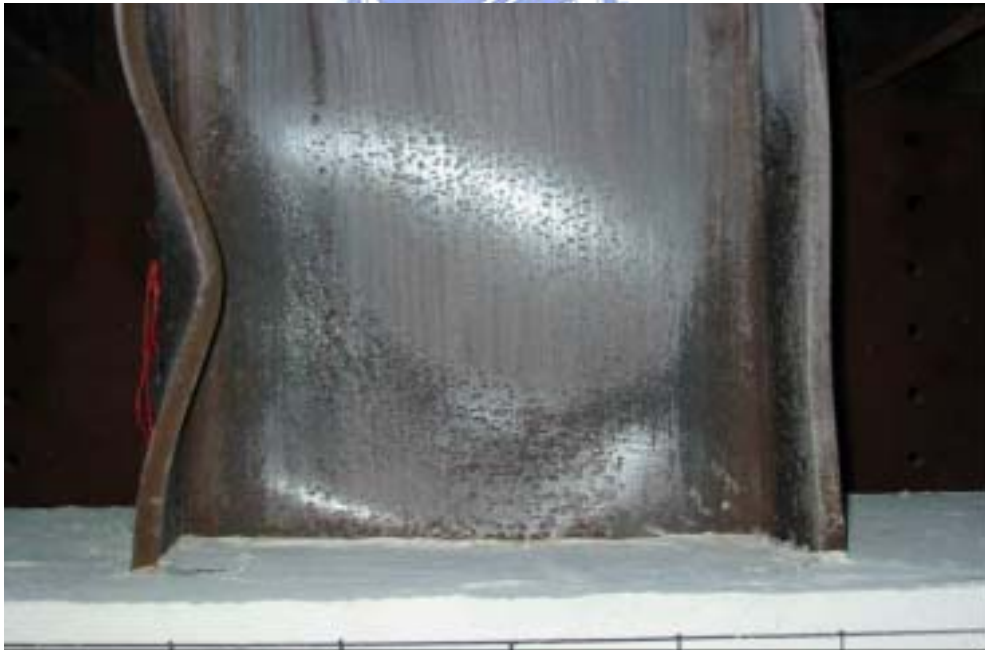
(b) 位移 9\Delta y 時( Story Drift Angle \theta_t = 4.30\% \text{ rad} , Beam Plastic Rotation \theta_{bp} = 2.82\% \text{ rad} )
