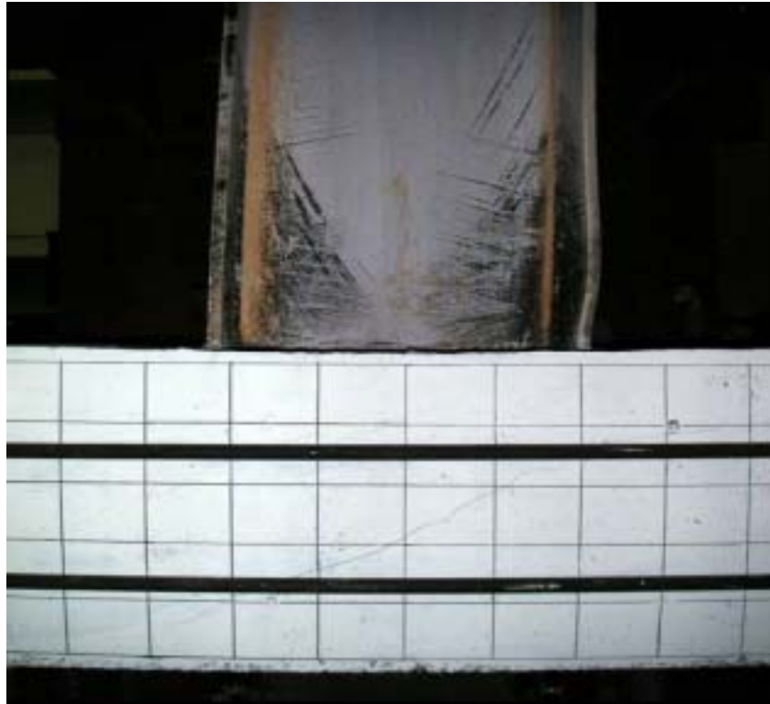
(a) 位移 7\Delta y 時( Story Drift Angle \theta_t = 3.34\% \text{ rad} , Beam Plastic Rotation \theta_{bp} = 2.12\% \text{ rad} )
