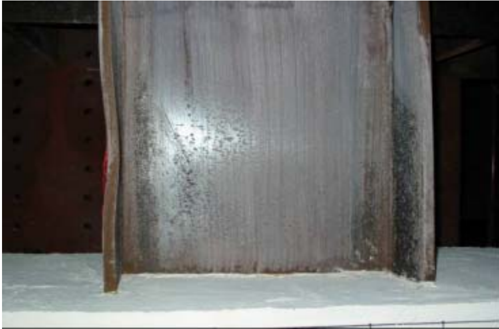
(a) 位移 8\Delta y 時( Story Drift Angle \theta_t = 3.82\% \text{ rad} , Beam Plastic Rotation \theta_{bp} = 2.14\% \text{ rad} )
