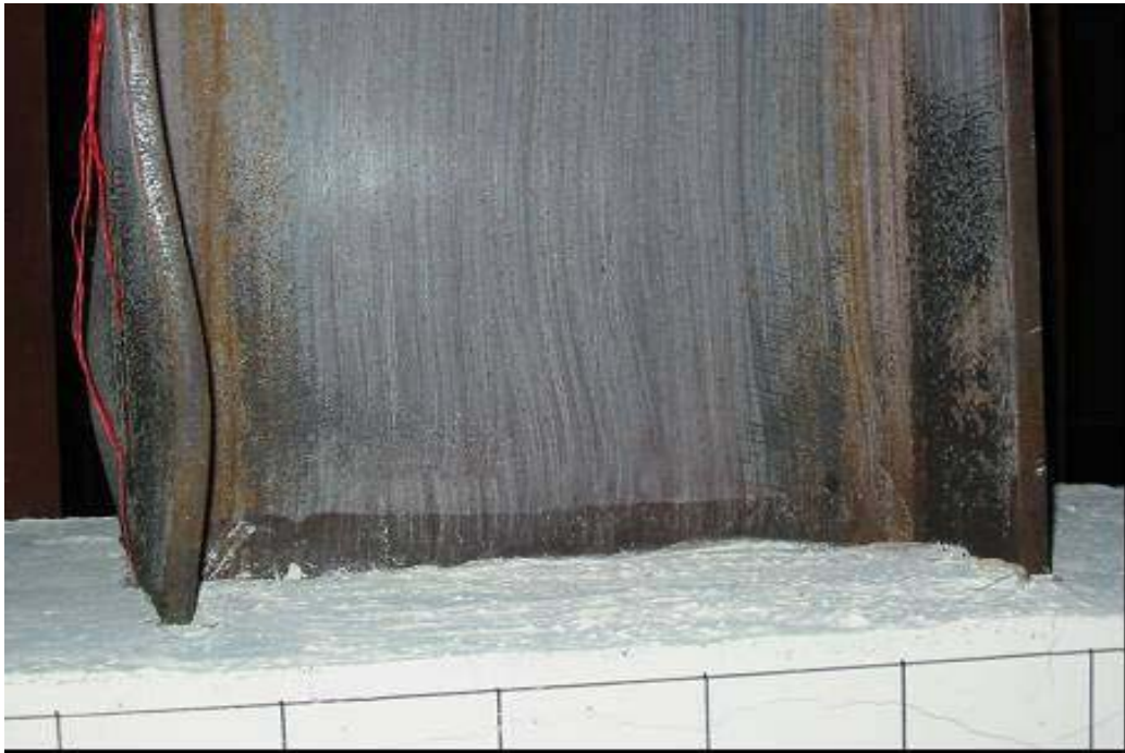
(a) 位移 7\Delta y 時( Story Drift Angle \theta_t = 3.34\% \text{ rad} , Beam Plastic Rotation \theta_{bp} = 1.74\% \text{ rad} )
