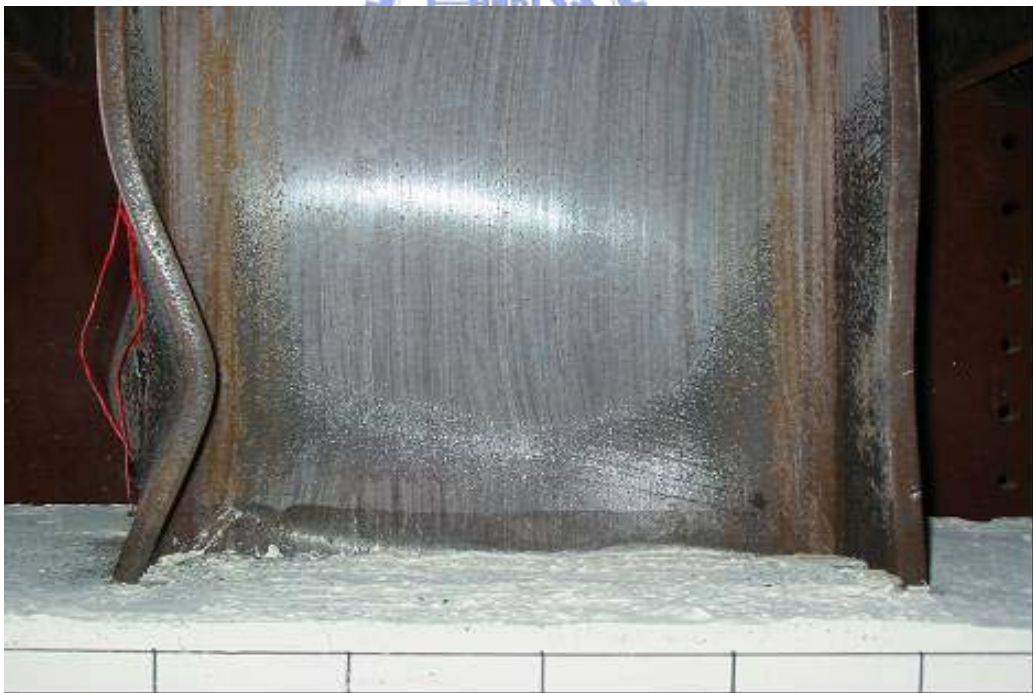
(b) 位移 8\Delta y 時( Story Drift Angle \theta_t = 3.82\% \text{ rad} , Beam Plastic Rotation \theta_{bp} = 2.15\% \text{ rad} )
