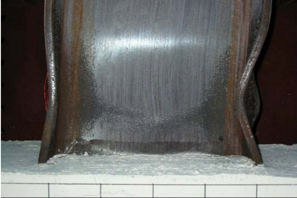
(c) 位移 9\Delta y 時( Story Drift Angle \theta_t = 4.30\% \text{ rad} , Beam Plastic Rotation \theta_{bp} = 2.65\% \text{ rad} )
