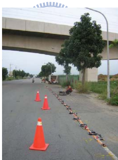
Fig. 3-19 The land streamer developed at NCTU
