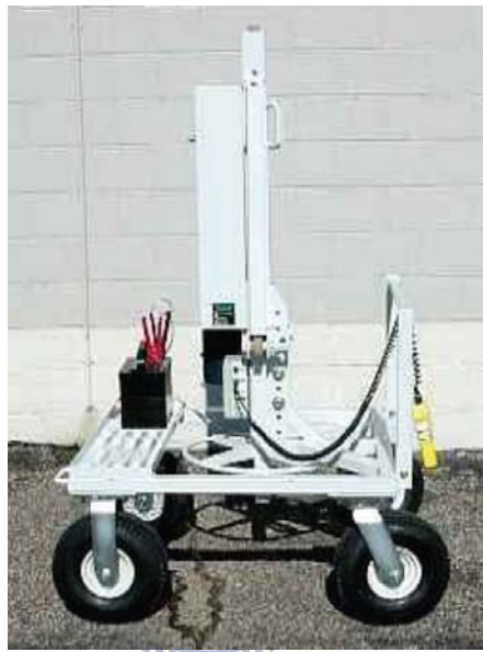
Fig. 3-13 Electrical operated seismic source ESS100SC
