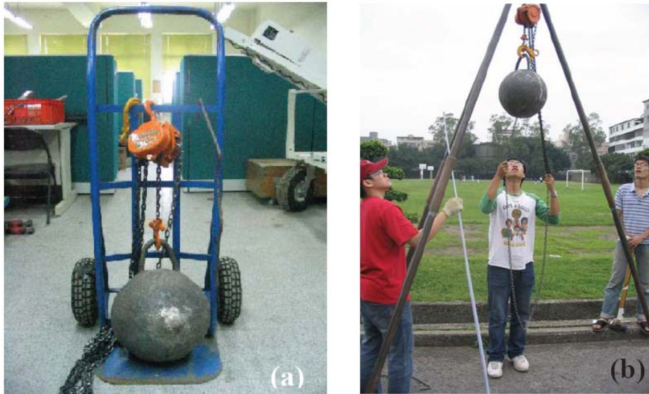
Fig. 3-14 New developed weight-drop seismic source
