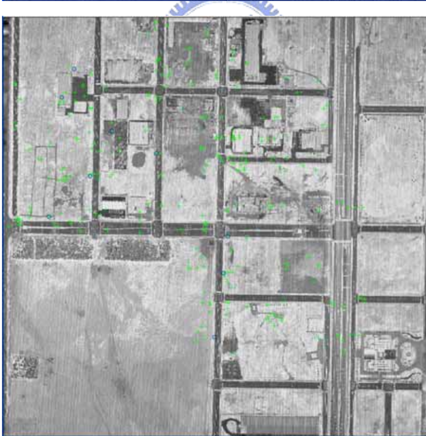
Figure 5.9: The matched points in two overlapping strips from intensity image
