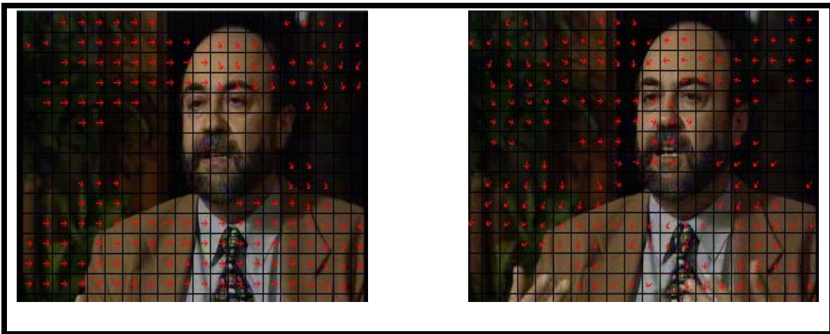
Fig. 3-3 extracted motion vectors from video stream “interview”
