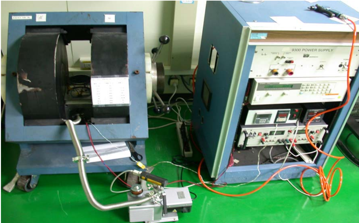
Fig. 3-5 Image of the field annealing setup. This system has an electromagnet and a vacuum anneal chamber, and the working pressure is 1 \times 10^{-3} Torr.
