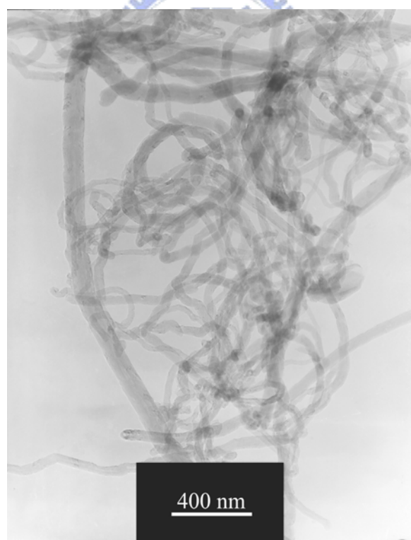
Fig. 4-6 Low magnification TEM image of purified MWCNTs.
