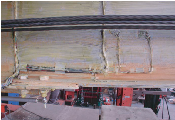
(a) Specimen 1 beam yielding (5% drift).
