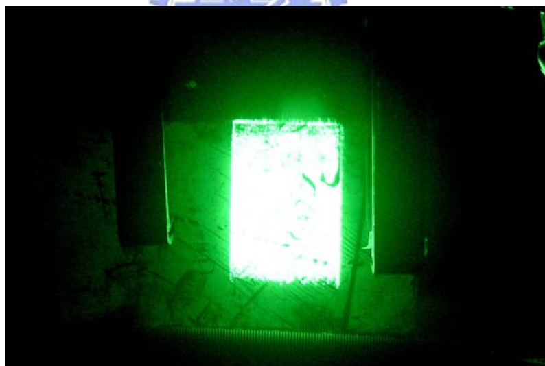
Fig. 4.27. Emission image at applied field 5.5 V/μm for diode testing
