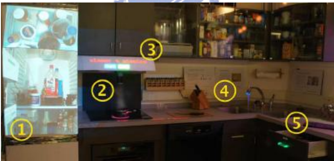
Figure 2-7 Augmented Reality Kitchen: (1) information projection on the refrigerator; (2) the range; (3) the cabinet; (4) the faucet; and (5) drawers.
